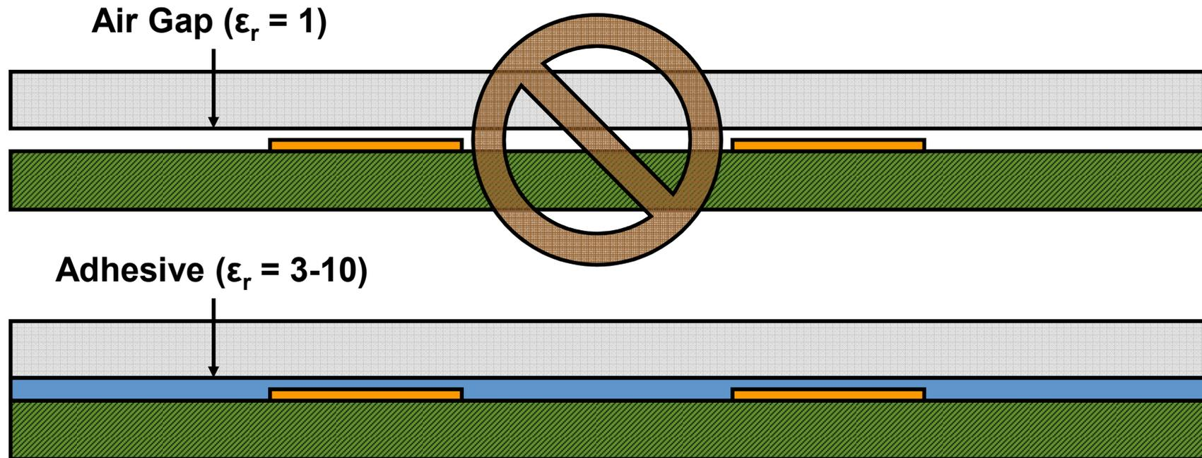
Air gaps decrease sensitivity ( $C_{\text{FINGER}}$  and  $C_{\text{BODY}}$ ) by **3-10x!**
