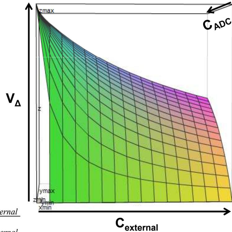
$$V_{\Delta} = \frac{C_{ADC} - C_{external}}{C_{ADC} + C_{external}}$$
